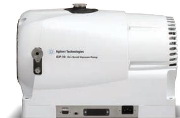
The IDP-10 oil-free vacuum pump delivers pumping speeds of 170 L/m (10.2 m<sup>3</sup>/hr). It is compatible with Agilent 7000 and 7010 Series triple quadrupole GC/MS systems.
