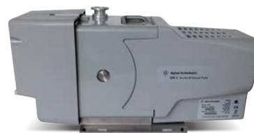
The IDP-3 oil-free vacuum pump is MSD qualified and delivers pumping speeds of 60 L/m (3.6 m<sup>3</sup>/hr). It is compatible with Agilent 5973, 5975, and 5977 GC/MSD systems.
